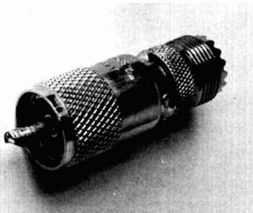
fig. 11. The completed range extension assembly.
